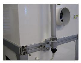
The cable is installed on the rear side of the AS-One. It is connected in the lower part of the signal tower. The green cover must be removed by turning it from the black base. Then the cable is connected as indicated on the picture hereunder:
